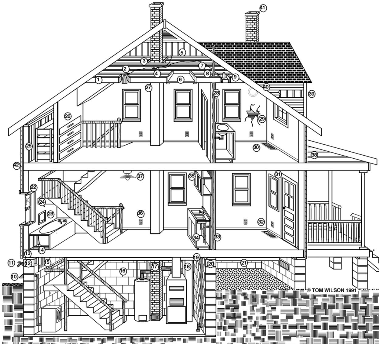
*Figure B-1. Graphic illustrating areas where retrofit air sealing and tactical insulation measures area are sometimes required.*
