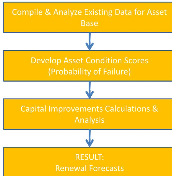
**Figure 1. Overall Approach to Condition Scoring and Subsequent Renewal Forecasting**
