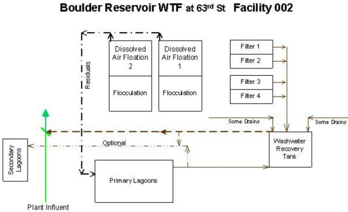
Figure 5-30: Existing Waste Impoundments at the Boulder Reservoir Water Treatment Facility
