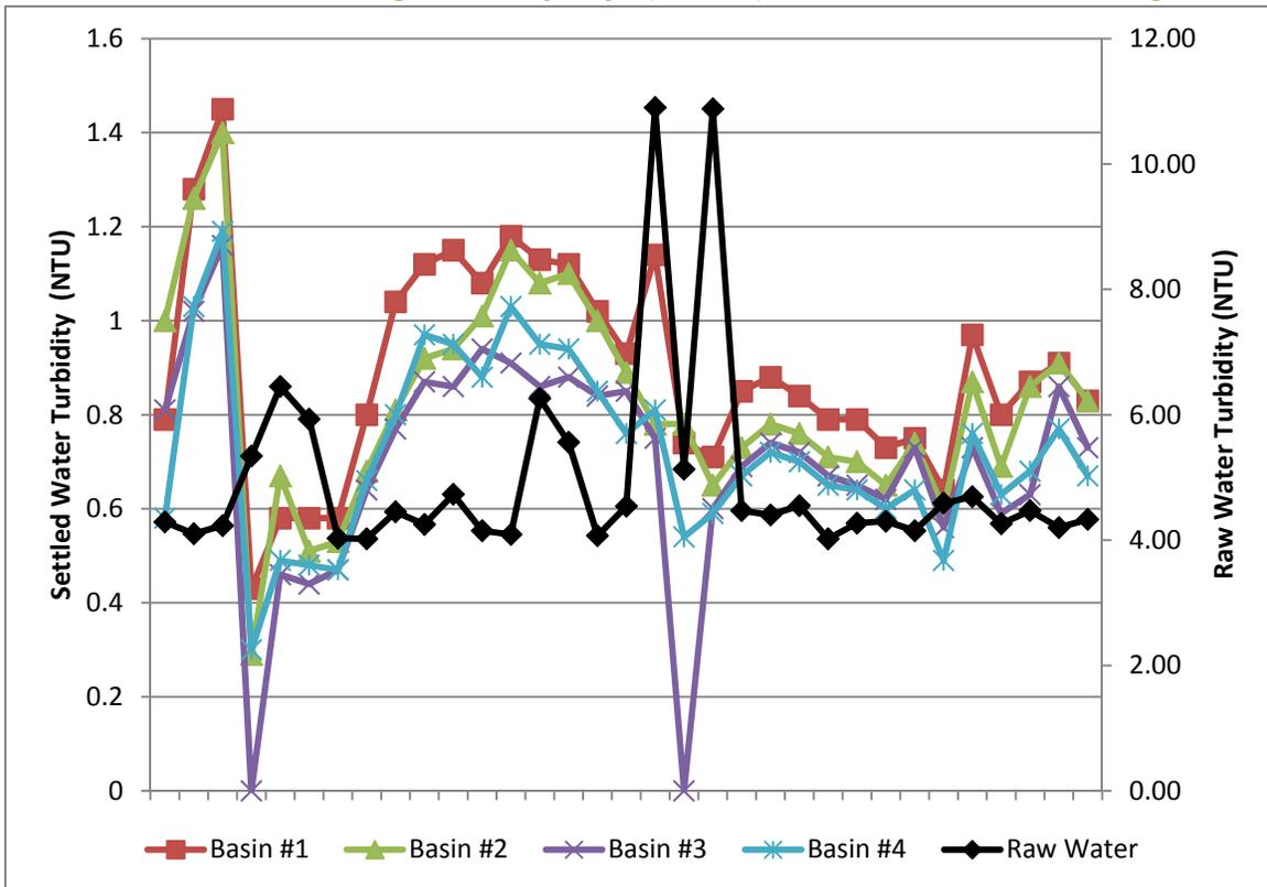
**Figure 5-12: BWTF Lakewood High Turbidity Days (> 4 NTU) Settled and Raw Water Average Turbidity**
