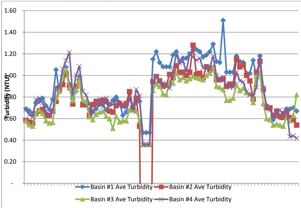
Figure 5-11: BWTF Barker High Turbidity Days (>4 NTU) Settled & Raw Water Average Turbidity
