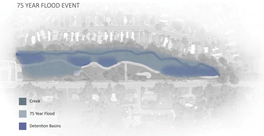
Similar to the 2013 flood, the entire site of Violet Park is prone to flooding. This flooding event is called a 75 year flooding event, where there is a 1 in 75 chance that this flooding event could happen. With these detention basins, and french drains, the surrounding neighborhoods are protected from this traumatic flooding event, and keeps the water within this site.
