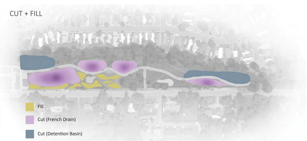
With the amount of water that can flood the site, there needs to be low points to collect storm water, as well as high points to allow for programs that cannot flood. By removing soil from the parts of the site that are detention basins, and french drains, it created low areas that allow for the storm water to be collected there. The high points can be created by taking the removed soil and "filling" it into these high points.
