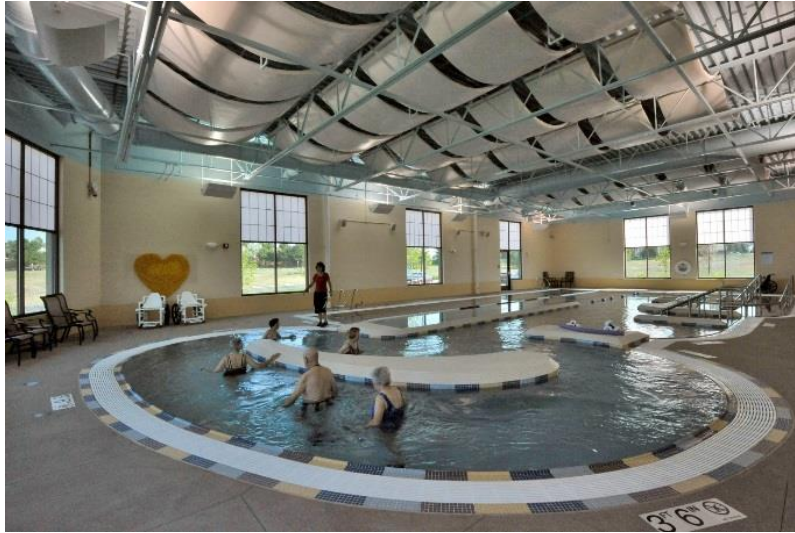
Photo 20 - Example of Best Practice of Acoustical Treatment PVC Encased Lapendary Baffles
