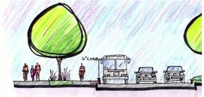
A narrow paved buffer separates the protected bike lane from the roadway, and a wide amenity zone with street trees is located between the protected bike lane and the multi-use path.
