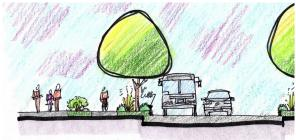
A wide amenity zone with street trees separates the protected bike lane from the roadway, and a narrower amenity zone is located between the protected bike lane and multi-use path.
