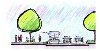
**CURBSIDE RAISED PROTECTED BICYCLE LANE** Separated from the sidewalk/multi-use path by an amenity zone. (Example cross section - Option 1)
