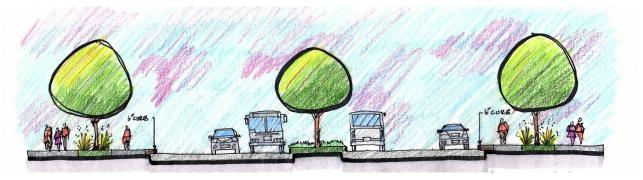
CENTER-RUNNING BRT - EXAMPLE CROSS-SECTION
