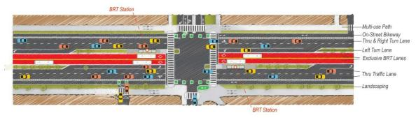
Alternative D: Center-running BRT in an exclusive transit lane with three general purpose lanes, an on-street bikeway, and a completed multi-use path
