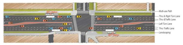
Alternative A: Enhanced bus in mixed-traffic with three general-purpose lanes and a completed multi-use path for pedestrians and bicycles
