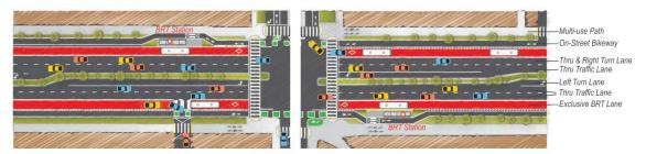
Alternative C: Center-running BRT in an exclusive transit lane with two general purpose lanes, an on-street bikeway, and a completed multi-use path
