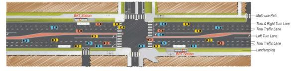
Alternative B: Side-running BRT in a semi-exclusive business-and-transit (BAT) lane (allows right turns) with two general purpose lanes, an on-street bikeway, and a completed multi-use path
