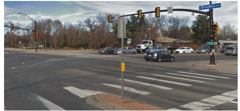
Full Traffic Signal at Intersection with Pedestrian Head Start is similar to the image above. The difference is that the light for the pedestrians turns white a few seconds earlier than the green light for cars.
